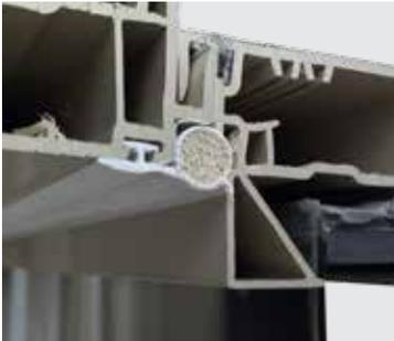
Bulb seals are seamless closed-cell compression seals that prevent water from penetrating the foam cell structure. Its extruded skin provides a unique UV resistant barrier with design features that enhance the weatherstrip's sealing performance.
