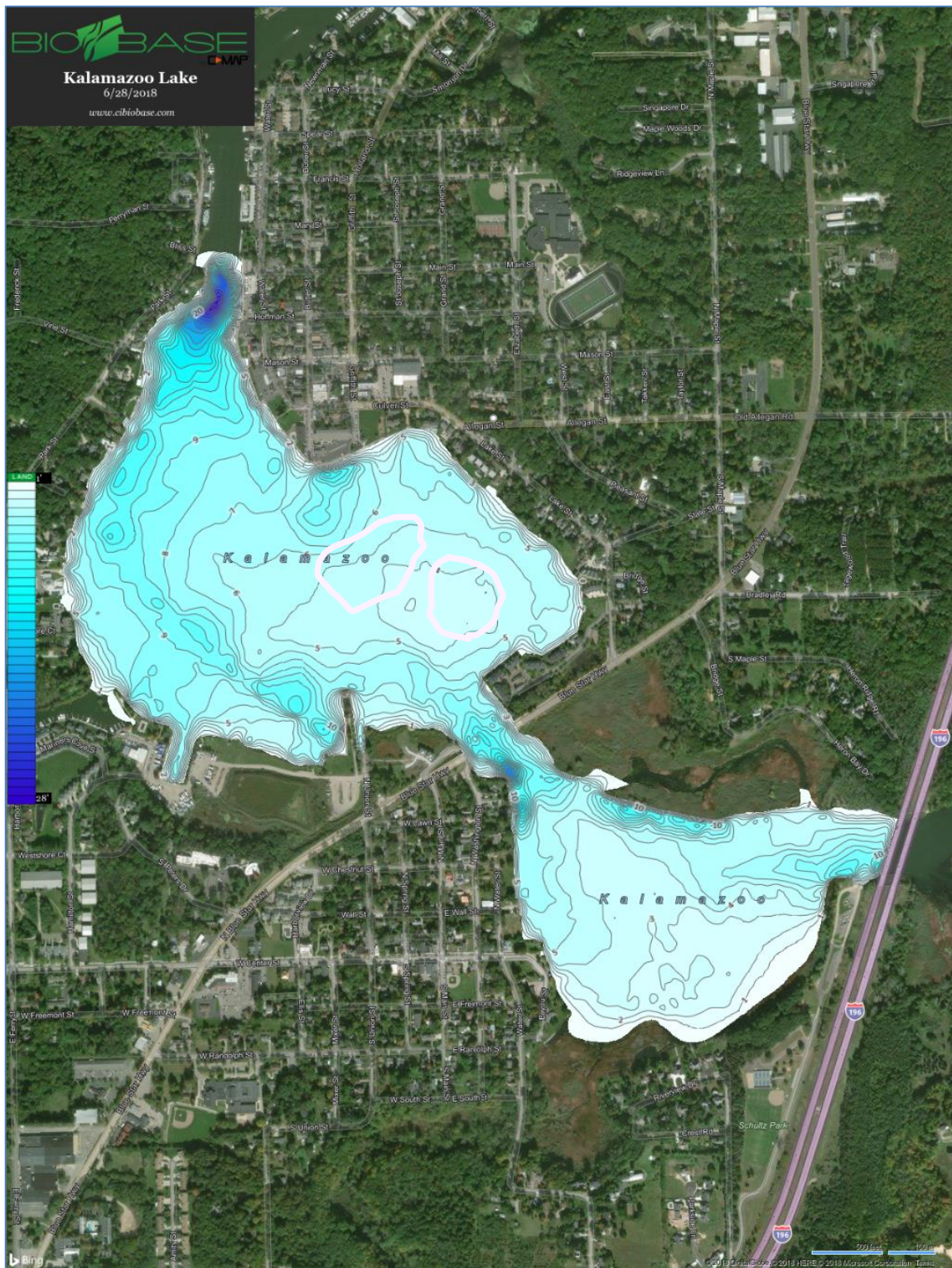
Figure 1. Kalamazoo Harbor Bathymetric Contour Map, Kieser & Associates, June 2018
